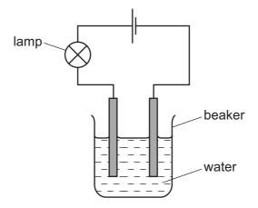
The lamp does not light when the beaker contains pure water.
